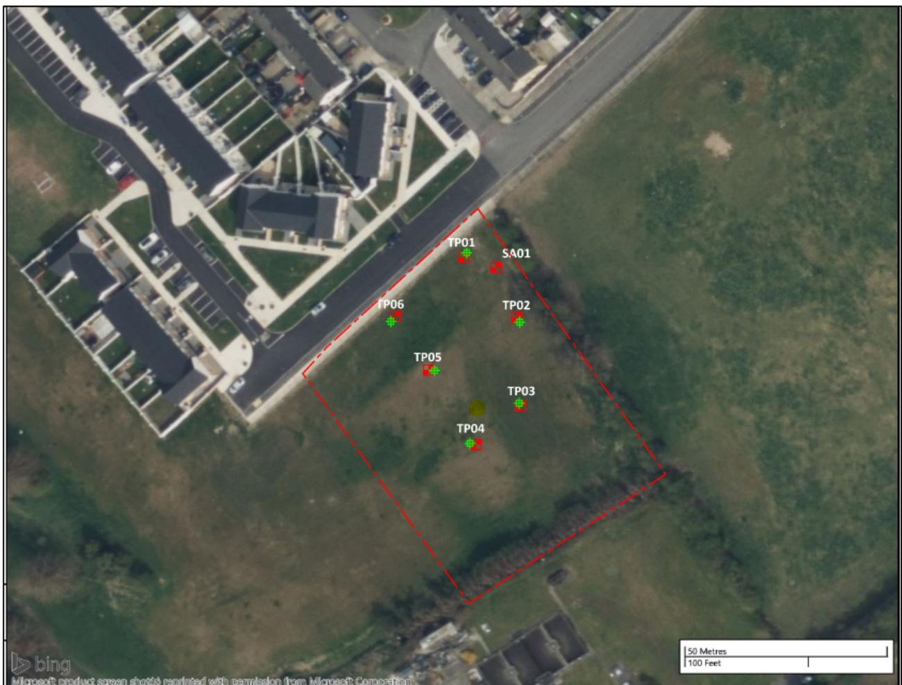
*Figure 5: Trial Pit and Dynamic Probe locations*
